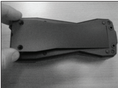
2. Remove the cover of the charging cradle.
